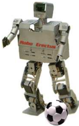
Figure 2.16: Robo-Erectus (RE) is a low-cost autonomous humanoid robot being developed at ARICC (the Advanced Robotics and Intelligent Control Centre) in the School of Electrical and Electronic Engineering, Singapore Polytechnic. The current challenge for the Robo-Erectus project is to develop a team of low-cost soccer-playing humanoid robots that are capable of walking, turning, crouching, and kicking a football past a goalkeeper into the goal.
