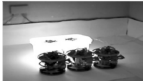
Figura 2.7. Robots modulares auto-reconfigurables Min-itans .
